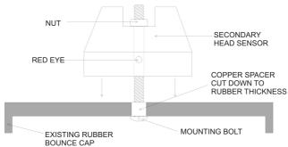
If mounting sensors with legs downards, a copper spacer must be used as shown below to prevent damage to sensor caused by over tightening the nut.
